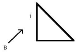
For the vertical side, the component of the magnetic field that is perpendicular to the wire would be given by Bcos(45), and for the horizontal side it would be Bsin(45). Since the sine and cosine of 45 are equal this distinction doesn't matter, but it might matter for a different problem so it's good to be aware of it.
