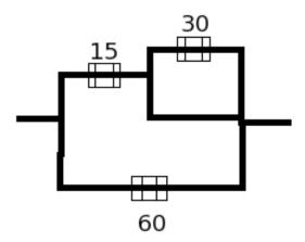
At this stage the current can get from "a" to "b" by travelling through either the 15 ohm resistor or the 60 ohm resistor. It does not need to go via the 30 ohm resistor at the top right. Which means that for all intents and purposes we can ignore it. So now we really have a simple parallel circuit with resistors of 15 and 60 ohms, and an equivalent resistance of 12 ohms.
