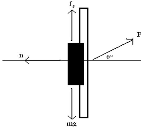
As always, it's best to put all your force vectors into their x- and y-components (if they aren't already) so we should break apart the applied force,  $F$ , into its y-component,  $F \sin \theta$ , and its x-component,  $F \cos \theta$ .
